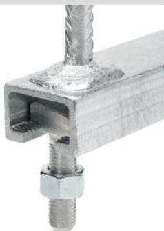
Anchor channels JXA-PC W 53/34 with JORDAHL® toothed T-bolt JXB
