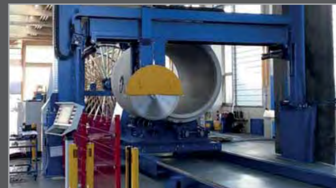
Special machine type PSF for sawing and milling of concrete pipes
