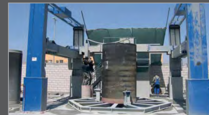
Special machine type VFM for vertical milling of concrete pipes
