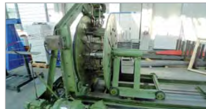
The first mbk cage welding machine
